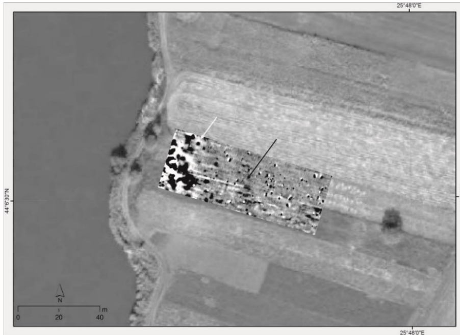
Fig. 10. The map of the magnetometric scan (the black arrow indicates the delimitation ditch; the white one indicates the positive anomaly verified by coring Sc5).
